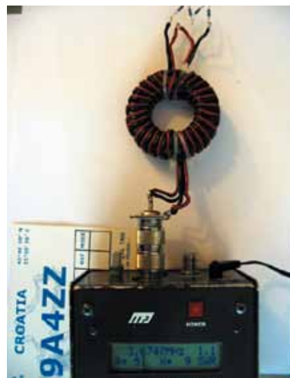
Slika 2b. TLT Guanella BALUN 1:4 (50:200 \Omega )
