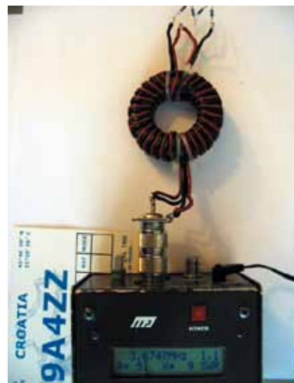
Slika 2b. TLT Guanella BALUN 1:4 (50:200 \Omega )
